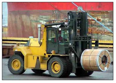
forklifts with diesel oxidation catalysts (DOCs). The DOCs are designed to reduce diesel pollution through a retrofit of the diesel exhaust systems. The DOCs are expected to reduce vehicle hydrocarbon emissions by 50%, monoxide emissions by 40% and particulate matter emissions by 20%.
